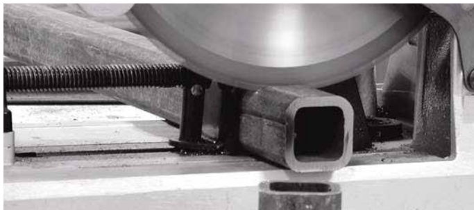
Carbide-Tipped Blades make Virtually Spark-Free Cuts
